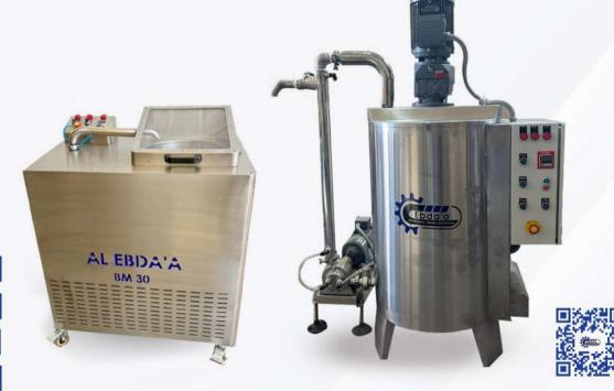
A cylindrical grinding machine. Available in many sizes (30,100, 250, 500, 1000) KG The wall is heated with a double jacket system with hot water by means of electric heaters Grinding is done by means of steel balls of different quantities and diameters
